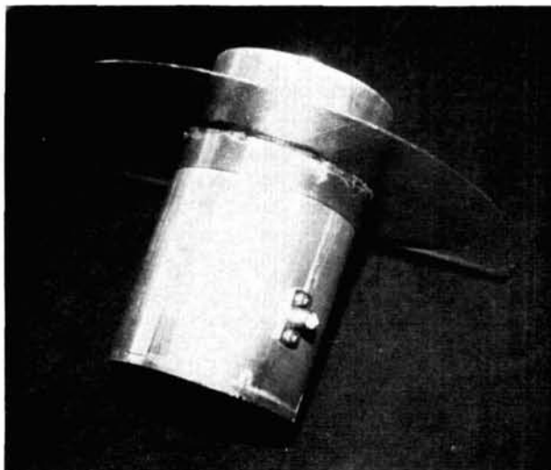
The flat disc rf choke is very effective in reducing back radiation and providing a better impedance match. VSWR measurements show that the best impedance match occurs when the choke is located at the best gain position. Details for adjusting the choke are given in the text.
